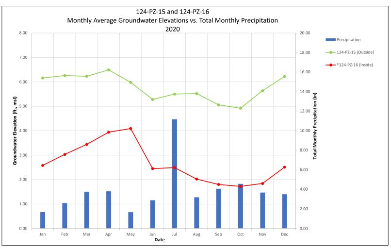
\*Based upon comparison to manual reading (3.85ft/ft on 6/16/20), PZ-16 data suspect for June. Datalogger sent back to manufacturer for calibration, replaced for July, and reporting accurately based on comparison with manual readings
