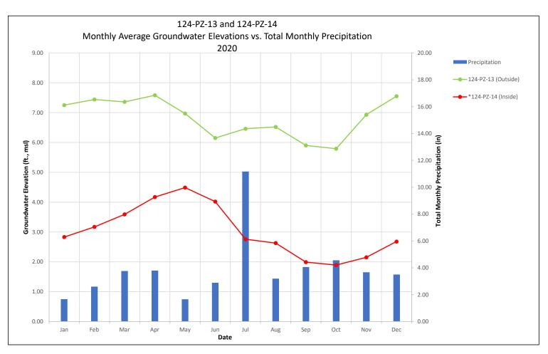
\* Due to extended pumping of the SA-6 South CGWES extraction pump for the Deferred Area Remedy, groundwater level in PZ-14 dropped below the elevation of the datalogger from 10/1/20 - 10/19/20. The elevation of the datalogger was 2.60 ft. Datalogger was lowered to compensate for low water level on 10/19/20.
