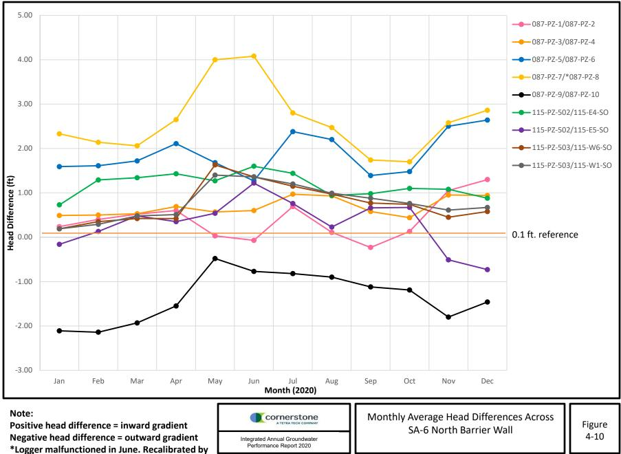
\*Logger maifunctioned in June. Recallb manufacturer and reinstalled in July.
