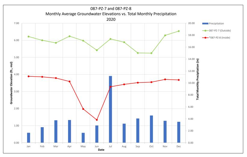
\* Based upon comparison to manual reading (3.08ft/ft on 6/16/20), PZ-8 data suspect for June. Datalogger sent back to manufacturer for calibration, replaced for July, and reporting accurately based on comparison with manual readings
